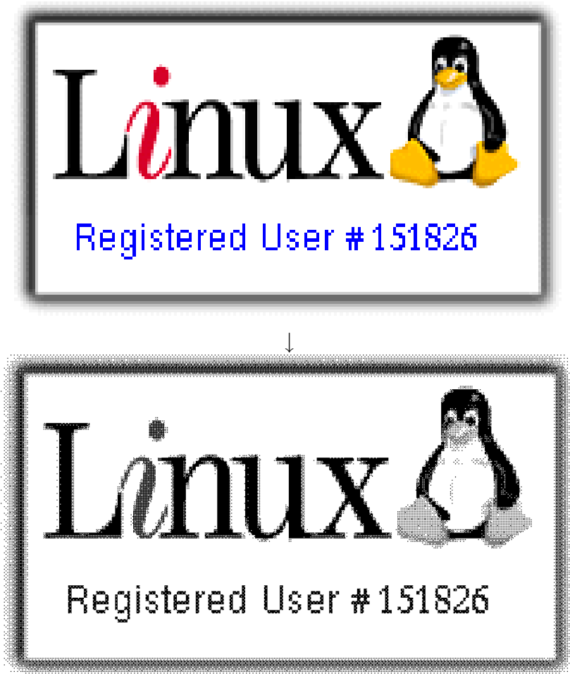
Figure 7: Black and white dithering. The colours and shades of the top picture are reduced to patterns of black dots in the bottom picture.
